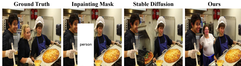
Figure 5: Visualization of image inpainting on COCO. Due to the existence of multiple people, Stable Diffusion cannot properly deal with the inpainting request, while GEODIFFUSION solves by successfully understanding location of missing areas thanks to the text-prompted geometric control.
